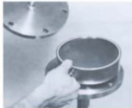
3. Remove the driver lid and driver housing.
