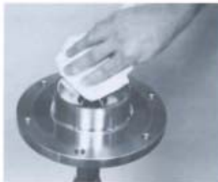
5. Clean the horn body and reassemble.
