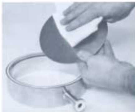
4. Clean the diaphragm and driver housing.
